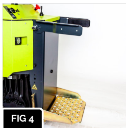
FIG 4 The safety rails locked in the raised position.
