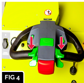
FIG 4 Traction paddles. Used to drive the truck.
