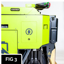
FIG 3 The safety rails in the lowered position.
