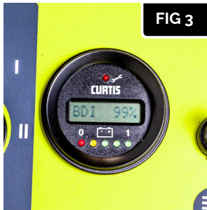
Multi function display. Battery discharge and fault codes indicator.
