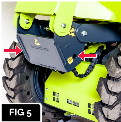
The anchor point locations on both sides of the crank.
