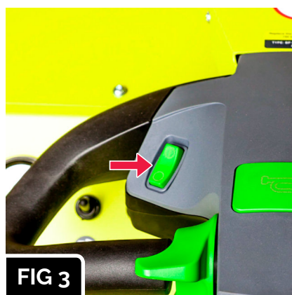
FIG 3 The location of the flashing beacon and motion buzzer switch on the tiller head.
