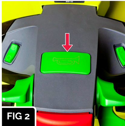
FIG 2 Horn switch. Pressed IN will sound horn.
