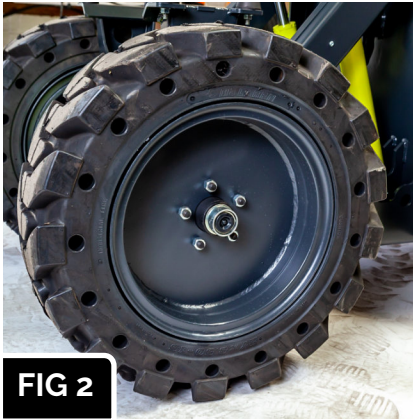
FIG 2 Check the front wheel retaining wheel nuts. If loose, tighten to the correct specified torque settings.
