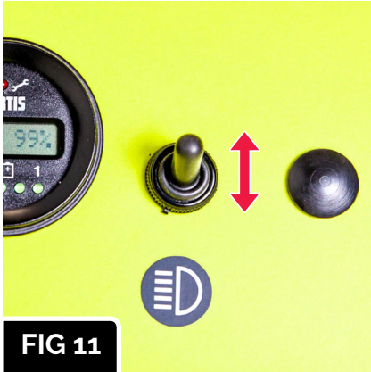
FIG 11 Ensure the light switch is working correctly. If applicable check the remote control switch.
