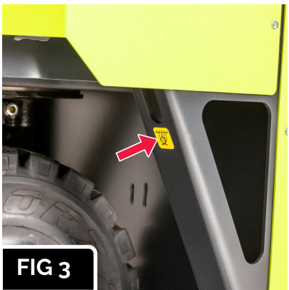
The anchor point locations are identified by this symbol.
