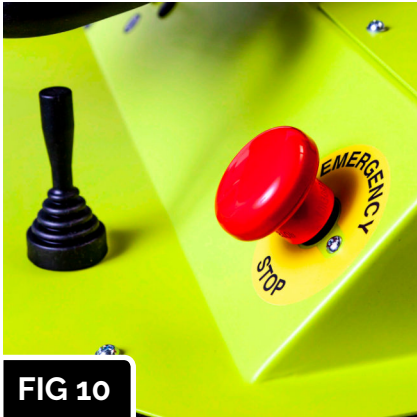
Check the emergency Stop button. When pressed in shuts machine down.
