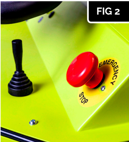
FIG 2 Emergency stop button Press the Emergency stop button to immediately interrupt all powered functions. Use the Emergency stop function if the control, driving or skip functions do not respond normally to operator commands. Use the Emergency stop as a service brake to secure the Truck when parked. To operate, the emergency stop button must be pulled up to the ON position before turning the key. If the emergency stop button is NOT in the ON position electrical power will not be transmitted to the Truck and the machine will fail to start.
