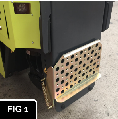
FIG 1 The platform in the raised position.
