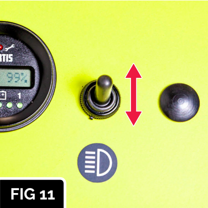
Ensure the light switch is working correctly. If applicable check remote control switch.
