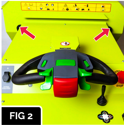
The two lifting point locations on the truck.
