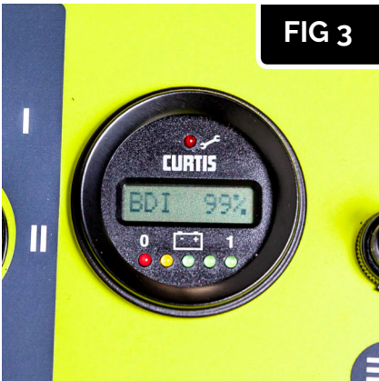
FIG 3 Multi function display Displays battery discharge (BDI), hour meter, trac hour and error messages. Error codes and troubleshooting can be found in the troubleshooting section of the Owners Manual.
