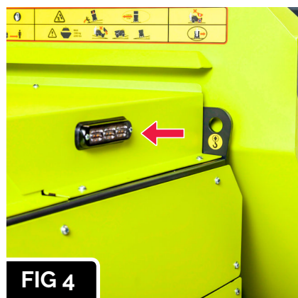
FIG 4 The location of the flashing beacon light, one on each side of the machine.
