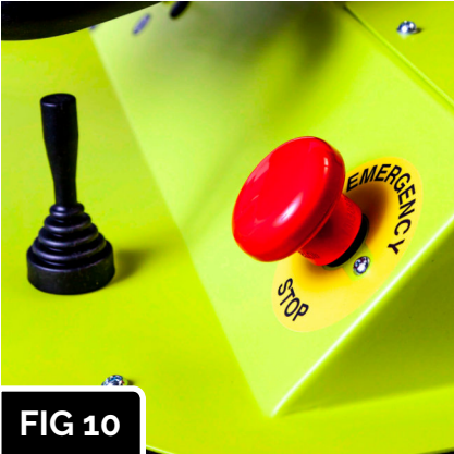
FIG 10 Check the emergency Stop button. When pressed down, shuts machine down.
