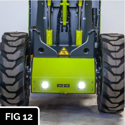
Ensure front facing lights are functioning and free from debris.
