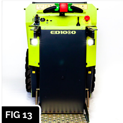
Ensure rear facing lights are functioning and free from debris.
