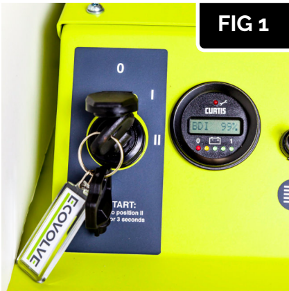
FIG 1 Key switch To start the Truck, make sure the Emergency stop is raised up, turn the key clockwise to position II and hold for 3 seconds to start the Truck.
