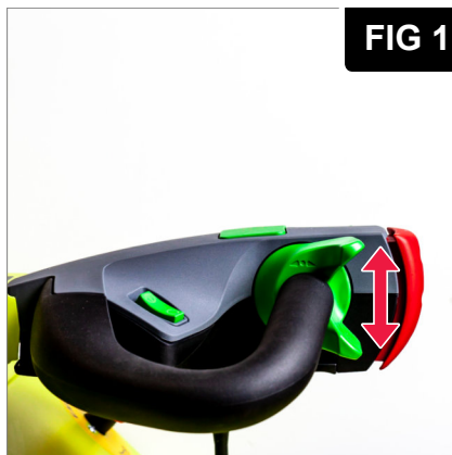
Traction paddles. UP =Forward DOWN = Reverse.
