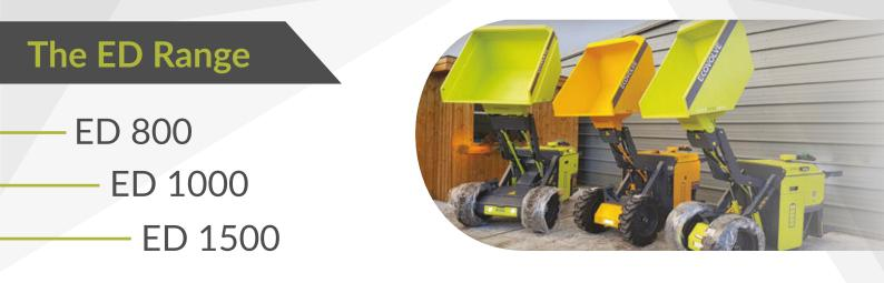
The Electric Dumper Range from Ecovolve is the worlds only fully electric hi-tip dumper. The dumpers are available in three different weight capacities - 800 kg, 1000 kg and 1500 kg skip. There are no fumes, no emissions, low noise and the steering system significantly reduces the risk of unwanted tyre marks. What's more is that the super elastic tyres eliminate the possibily of puncture, making the ED Range suitable for both indoors and out.
